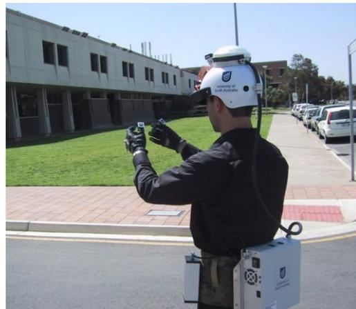
Figure 1. Tinmith augmented reality wearable computer system
