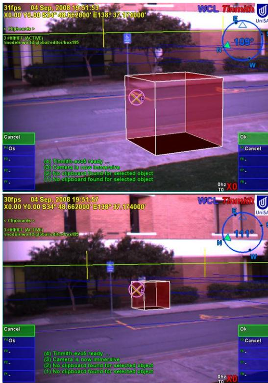
Figure 7: Ground plane translation of a virtual box. Top: before translation. Bottom: after translation.
