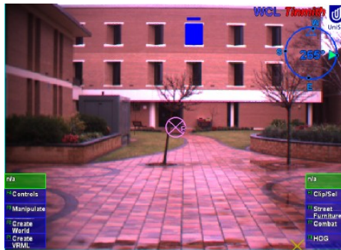
B: The view through the user's head-mounted display (blue boxes indicating distant virtual objects overlaying the physical window)
