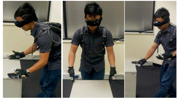
Figure 1: Modeling by measurements using ultrasonic gloves on a filing cabinet (subfigures - a. length, b. width, and c. height)
