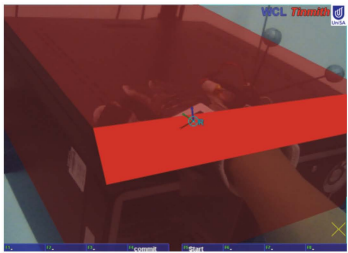
Figure 5. Chamfer technique is performed by directly touching the surface edges during manipulation
