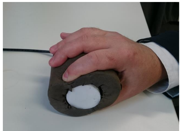
Figure 7 The horizontal grip with flexion of index finger to steer the car for FingerRacer
