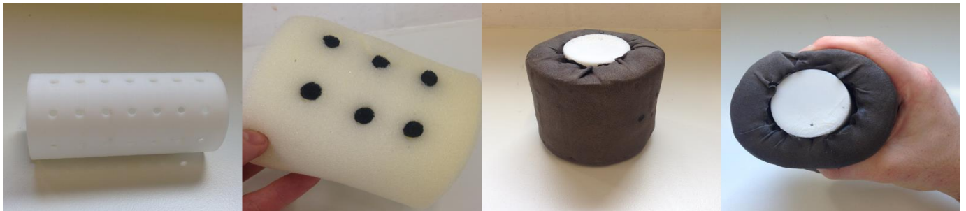
Figure 1 HandLog components and usage (from left): 3D printed core; foam sleeve (white) with embedded conductive foam (black) sensors; HandLog device with core and sleeve; Whole hand finger flexion gesture
