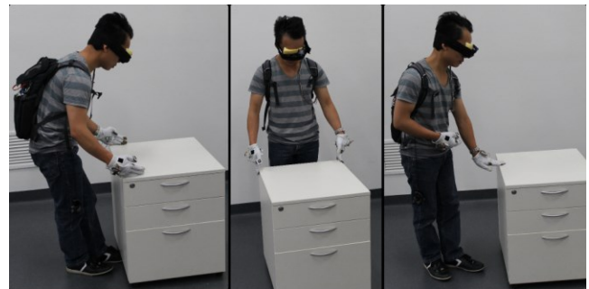
Figure 1: Modeling by measurements using ultrasonic glove and filing cabinet (subfigures - a. width, b. length, and c. height)
